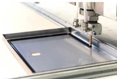
CNC machine for applying polyurethane gasket
