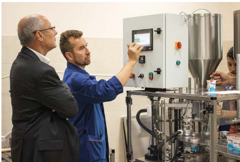
Testing the operation of the filling machine on the customer's container
