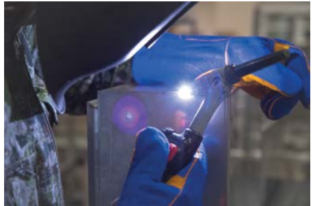
Argon welding process
